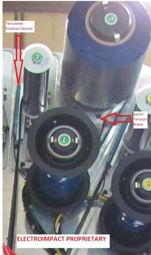
Figure 6 – AFP Head Spool, Backing Film Take-up & Dancer Configuration
